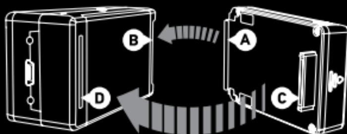
1. Slide hooked end of the BacPac (A) into the groove on the right side of the camera body (B).
