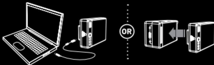
1. Connect the BacPac to a computer or any USB compatible wall or car charger such as a phone charger, etc. with the included USB cable.
