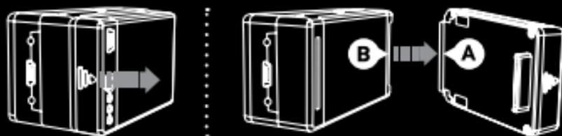
1. Pull back on left side of BacPac marked with the arrow to disconnect from the HERO bus port.
