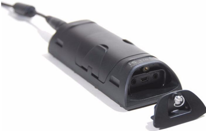
The Input/Output Port cover is located on the bottom of the POV.1.5
