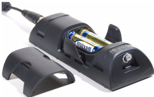
Back of the POV.1.5 with the battery compartment cover removed.
