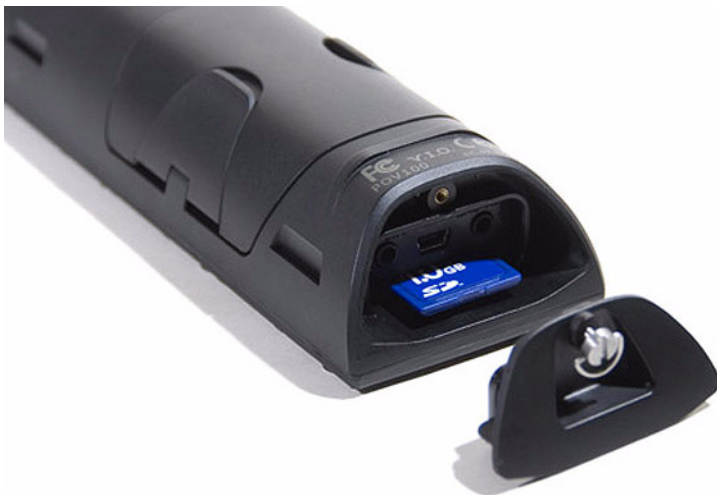
The bottom of the POV.1.5 with the SD card inserted
